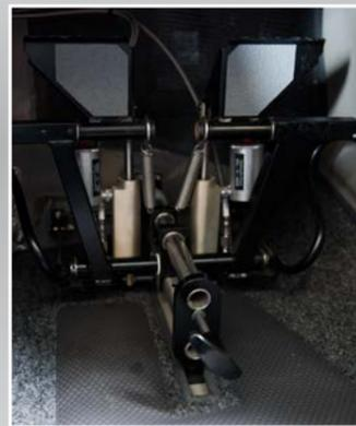
Electrically Operated Adjustable Rudder Pedals for Pilot and Copilot
